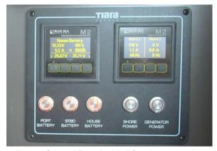
Power Control Panel with AC voltage monitor.
