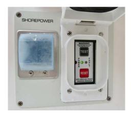
Shore power breaker and ground fault sensing module
