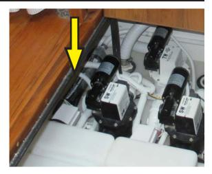
Waste tank vent air filter indicated by arrow
