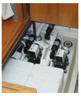
Tank vent filter, vacuum pumps, waste tank under the atrium floor hatch
