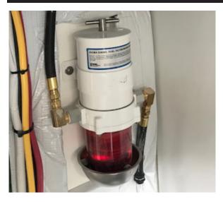
Fuel water separating filter (typical)
