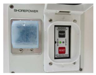
Shore power breaker (left) and ground fault sensing module
