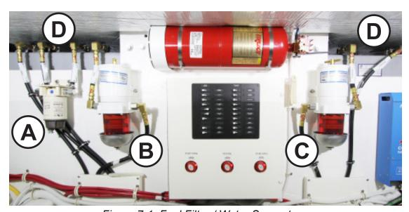
Figure 7-1: Fuel Filter / Water Separators:
