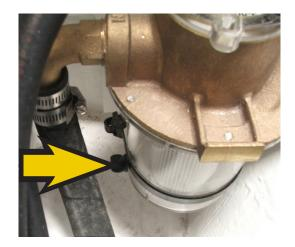
Figure 8-3: Raw water strainer sight glass drain plug.
