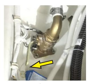
Figure 7-6: Seacock in closed position and secured with cable tie
