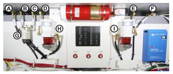
Figure 5-4: Fuel valves, lines and filters in the forward engine room
