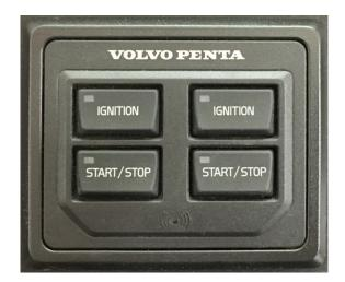
Figure 5-7: Volvo® e-Key control panel
