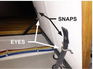
Figure 2-4: Hatch eyes and snaps
