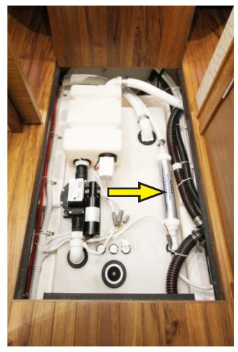
Figure 7-4: Top of the waste tank (located under the atrium floor hatch). The tank vent air filter is indicted by the arrow.
