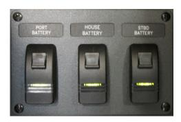
Figure 4-4: Battery Switch Panel
