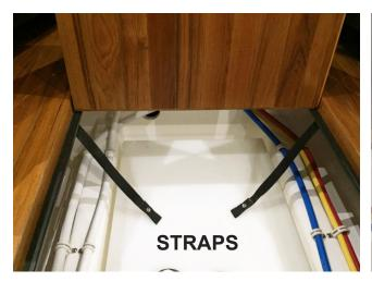
Figure 2-3: Hatch straps
