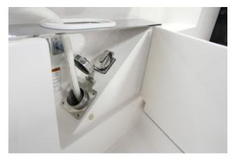
Figure 1-6: Aft shore power locker
