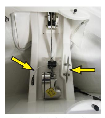
Figure 5-10: Anchor locker with windlass, mooring cleat and safety cable
