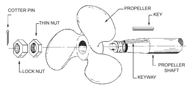
Figure 6-1: Propeller installation on shaft
