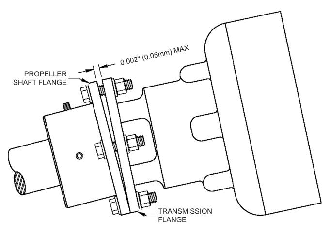
Figure 6-4: Transmission and propeller shaft flange alignment
