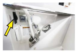
Figure 5-2: Aft port shore power locker and cable master switch
