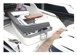
4. Continue rotating the cockpit to starboard and aft
