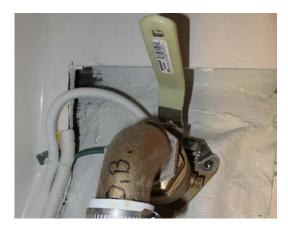
Waste discharge seacock, under cabin floor hatch
