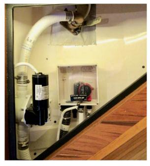
Waste pump (left), overboard discharge valve (top), shower sump box (bottom)
