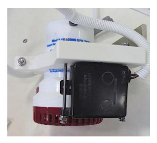
Typical bilge pump and float switch (right)
