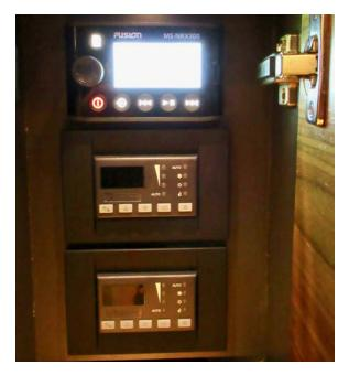
Climate control panels and stereo remote control panel, located in the starboard berth cabinet
