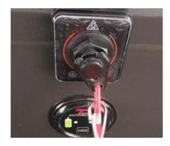
Engine stop switch and lanyard (typical)
