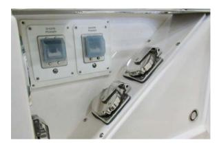
Main shorepower breakers and inlets in aft starboard shorepower locker
