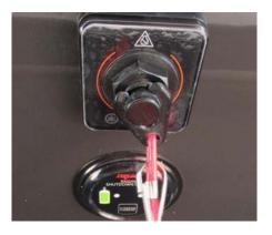
Engine stop switch and lanyard (typical)
