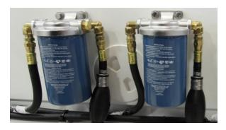
Gasoline fuel water separating filters (typical)
