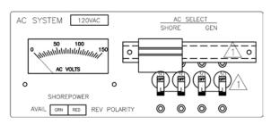
Detail of AC distribution panel schematic: shore power and generator power AC select switch and polarity indicator lights
