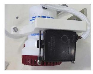
Typical bilge pump and float switch (right)
