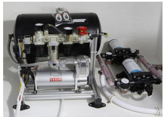
Figure 3-8: Air compressor and fresh water pumps
