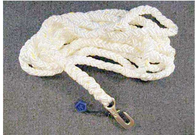
Figure 5-11: Snubber provided with optional all-chain rode
