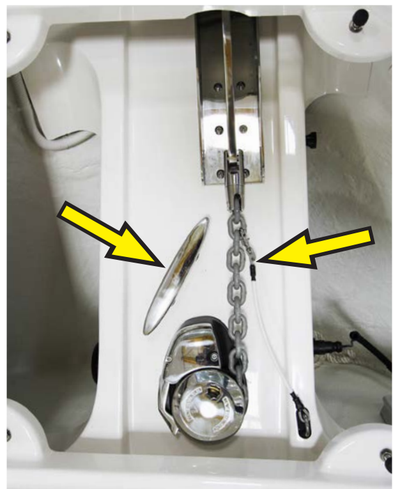
Figure 5-10: Anchor locker with windlass, mooring cleat and safety cable
