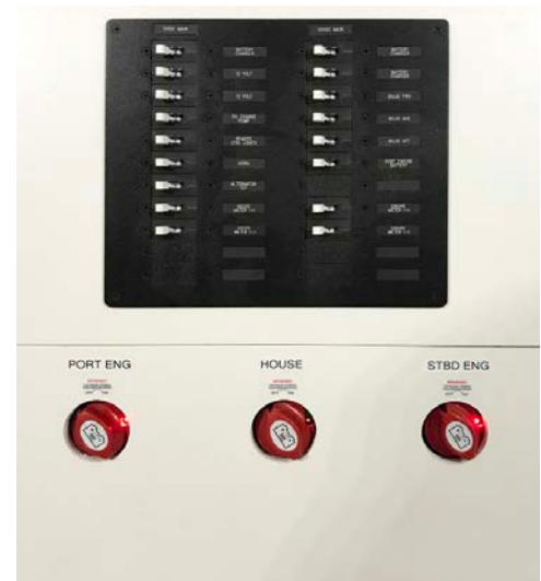
Figure 4-1: Master DC Panel
