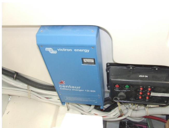
Figure 3-7: Port side forward engine room bulkhead. Battery charger (left), and port engine Cummins Vessel Interface Panel (right). In Zeus applications the Battery Charger is forward on starboard.
