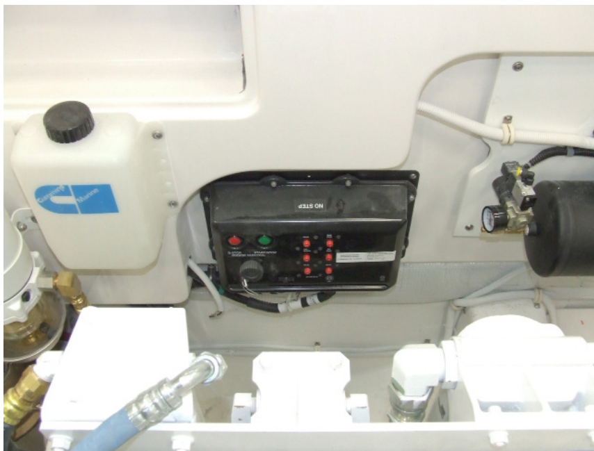
Figure 3-8: Starboard engine coolant overflow (left), horn compressor (right), Cummins panel (center).
