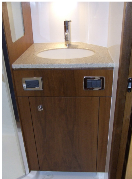
Figure 2-4: Lower vanity with Corian® countertop. Storage is below the sink. Read the literature provided by the manufacturer of the Vacuflush® toilet for operation details. Light and exhaust fan switches are in the forward face of the lower vanity.
