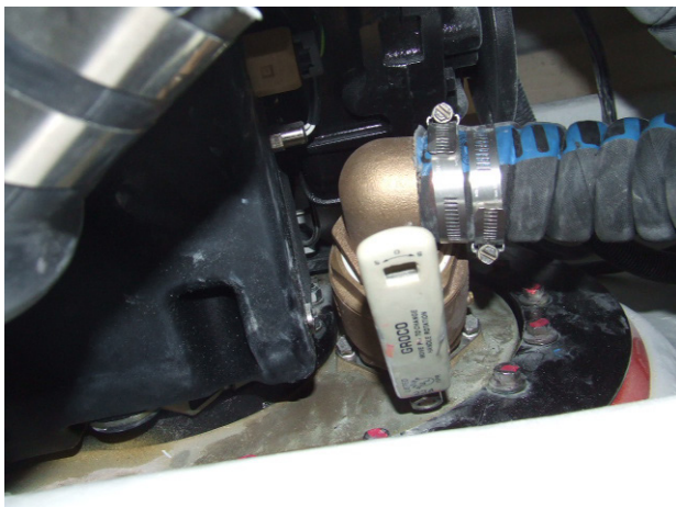
Figure 3-3: Zeus pod integral raw water seacock.
