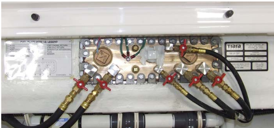
Figure 7-2: Fuel tank fuel valves, located below the aft centerline floor hatch in conventional drives or in the forward engine room with Zeus pod drive applications.
