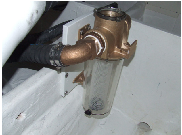
Figure 3-4: Port side raw water strainer shown in the aft bilge area. Zeus pod drive location only.
