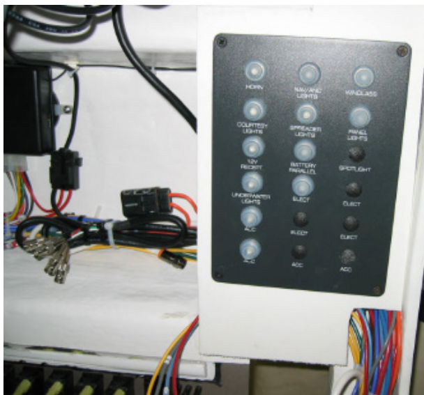
Figure 1-5: The helm breaker panel behind the console.
