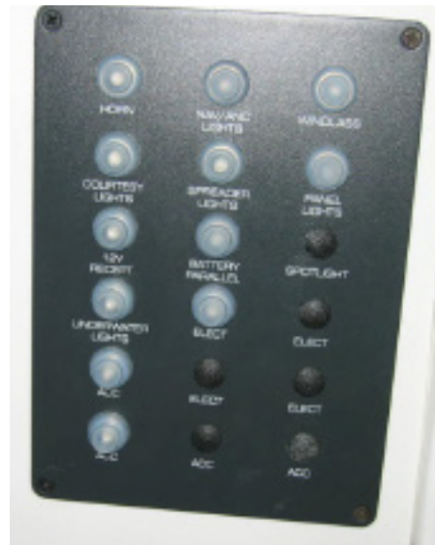
Figure 4-2: Helm Breaker Panel. behind the console.
