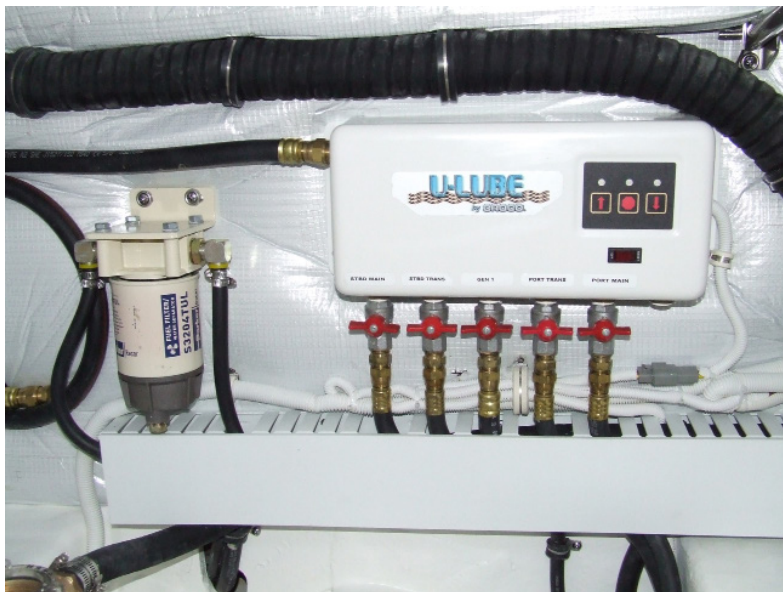
Figure 3-5: Aft of the starboard engine. Generator fuel water separator and oil changer. The oil changer is aft of the port engine in Zues applications.
