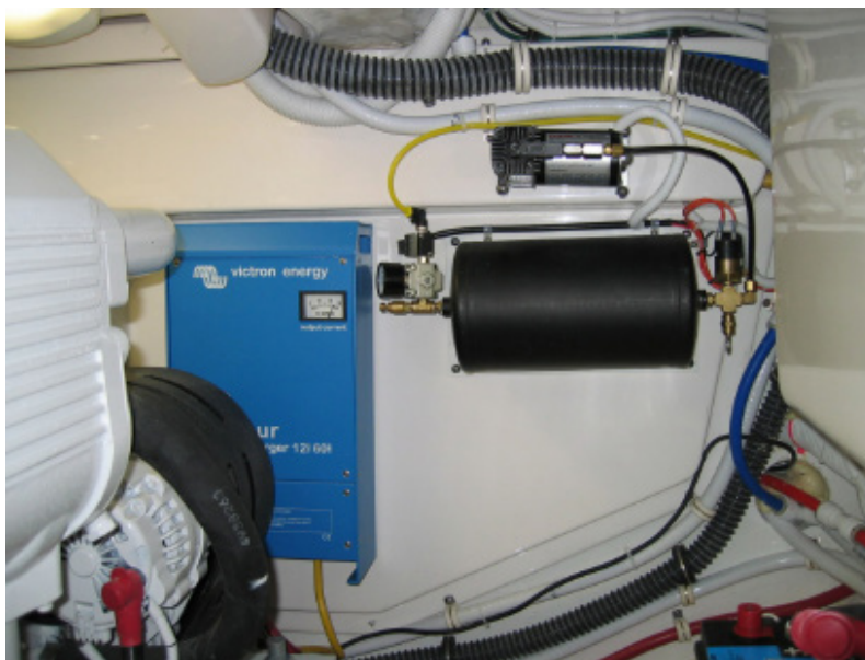
Figure 3-6: Starboard side forward engine room bulkhead. Battery charger (left), Horn compressor (right).
