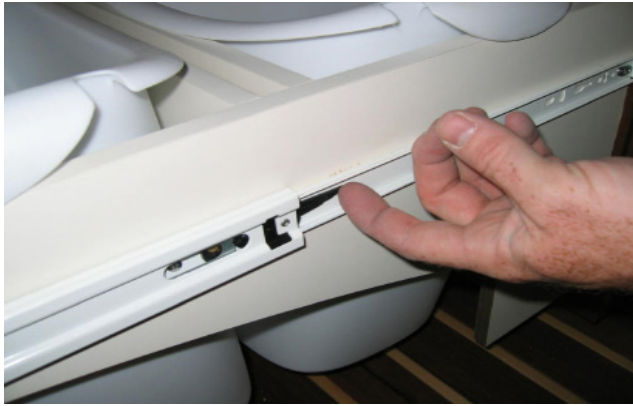
Figure 7-3: In the lower, aft, inboard galley, is the garbage can drawer. To pull out the drawer to its maximum open position toggle one side of the slide locks UP (shown with index finger) and the opposite side DOWN.
