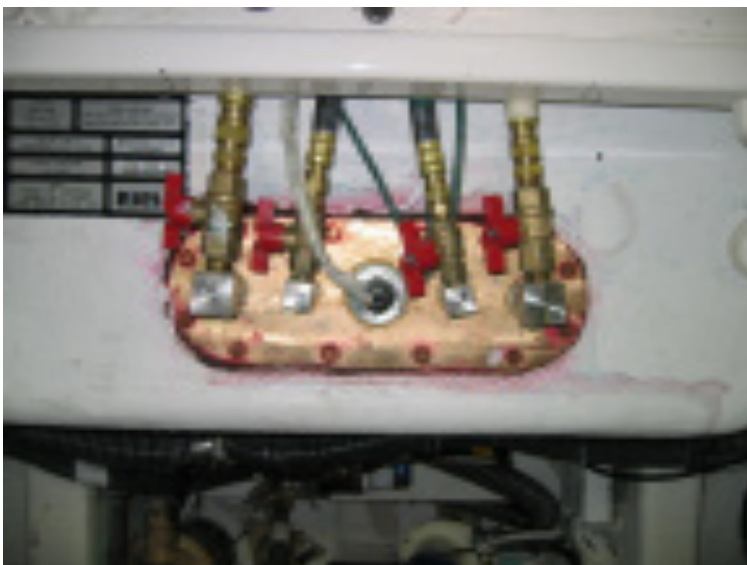
Figure 7-2: Aft fuel tank fuel valves, located below the aft centerline floor hatch.
