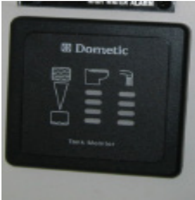
Figure 7-9: The Dometic® Tank Monitor Panel is located in the upper hullside cabinet above the dinette. Lights indicate the status of the waste tank and fresh water tank quantities. The graphic guide on the left of the panel indicates full or empty. A full head indicates a full waste tank and it should be promptly pumped out.
