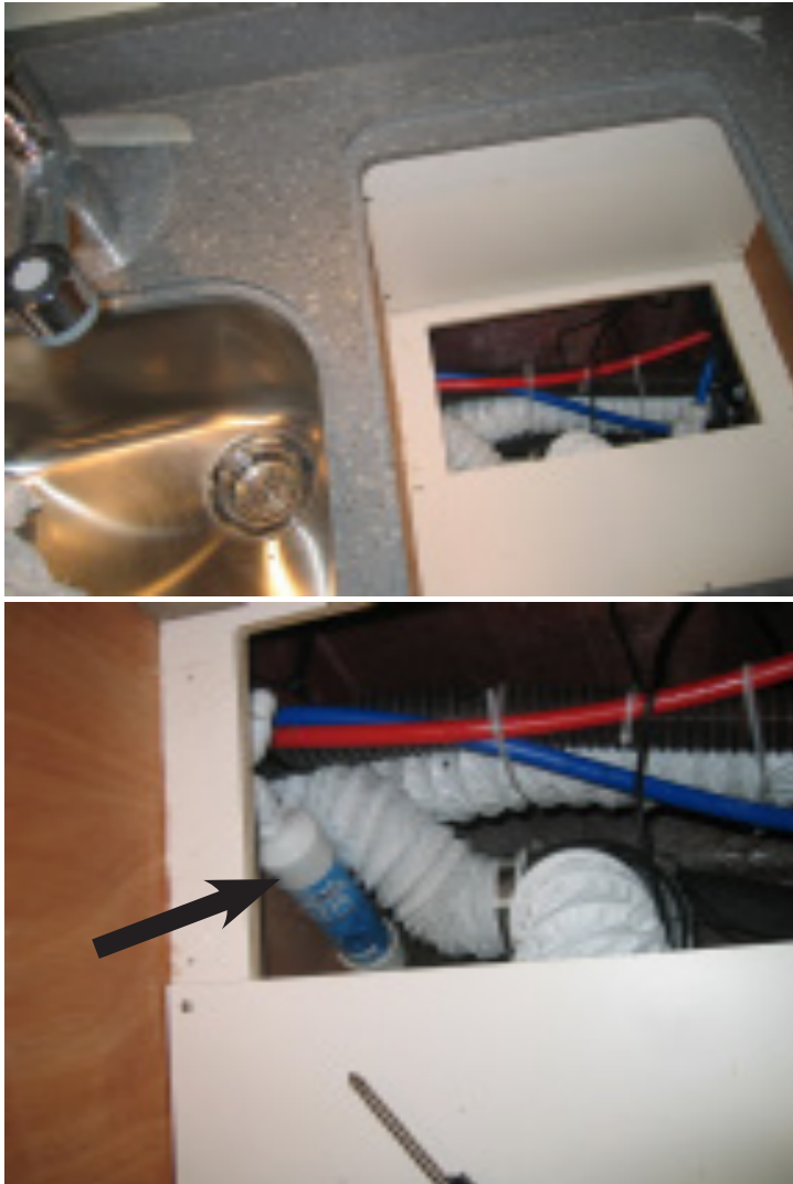
Figure 7-7: Access the galley inline freshwater filter by first removing the Corian® lid forward of the galley sink. Next remove the panel in the outboard storage compartment. The filter is on the aft side of the opening (arrow in lower picture).
