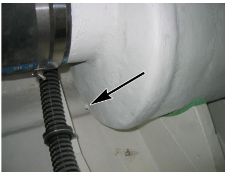
Figure 8-2: Port engine muffler plug shown. The muffler plugs are accessed through the port and starboard floor hatches.
