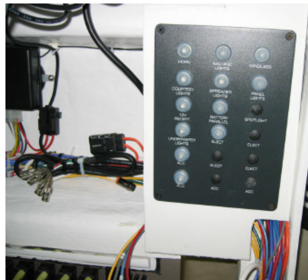
Figure 1-5: The helm breaker panel behind the console.
