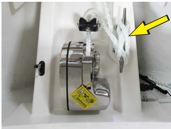
Windlass and anchor rode cleat (typical)
