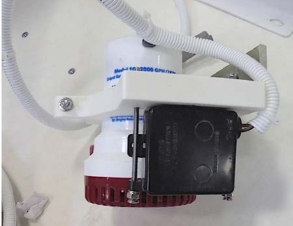
Typical bilge pump and float switch (right)
