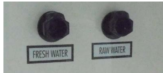
Optional fresh water and raw water washdown inlets, located under the helm seat
