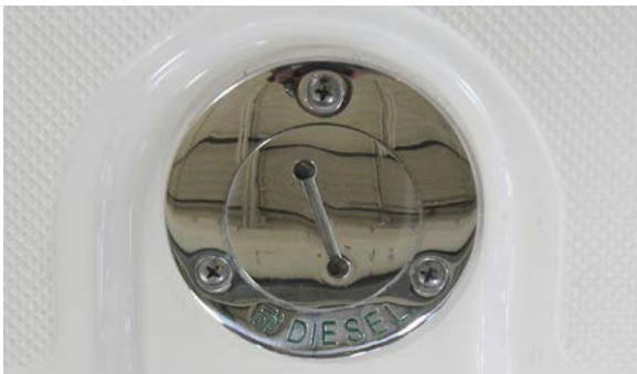
Diesel fuel fill
